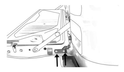
put damper bracket and tighten back the original bolt.
