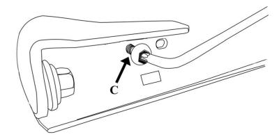
7. Attache tailgate bracket (A) on the truck tailgate bracket (B) Original bolt (C)
