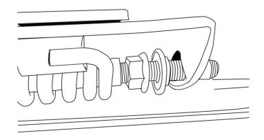
8.2 tighten nut (E) while holding the rod of the spring set with #6 wrench (F)
