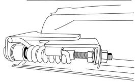
8.3 tighten nut (L) with wrench #12 (M) while holding nut (E) with wrench #12 (N)
