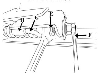
Make sure that the spring end (G) is slided in the bush (H) of the tailgate bracket
