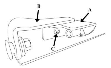
8. Assembly the spring set with tailgate bracket8.1 put spring set with tailgate bracket as below picture
