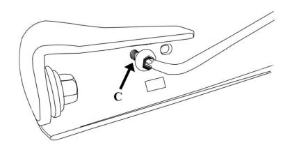
7. Attach damper to the tailgate by putting damper bracket (T) under tailgate sling bracket (U) and tighten together with original bolt (V) (W)
