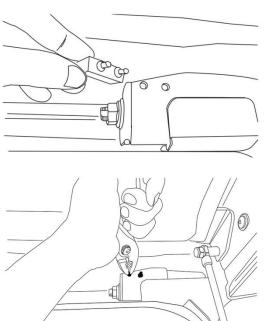
5. Attache spring pushing bracket (O) with the truck using original bolt (P). If the truck has stopping rubber, can put it back through hole (Q)
