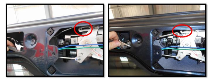
6. Release rods of the lock and central locking (as pictured)
