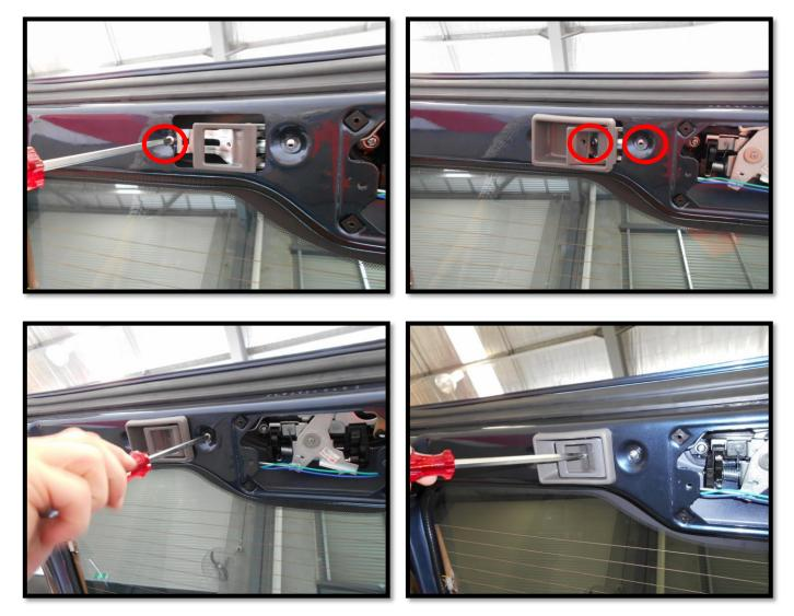
17. Replace the coverplate, tightening the 4 screws using a Phillips head screwdriver (as pictured)
