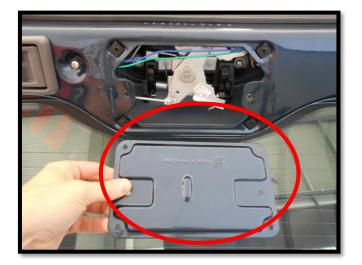
4. Remove internal handle by removing 2 screws using Phillips head screwdriver (as pictured)
