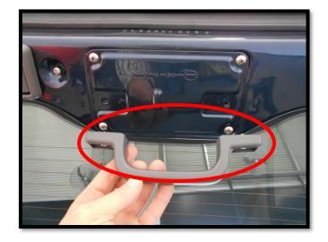
3. Remove the cover by unscrewing 4 screws using Phillips head screwdriver (as pictured)
