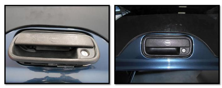
13. Replace and tighten the 2 screws using a Phillips head screwdriver to secure the handle (as pictured)
