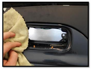
**10.** Apply the glue to a clean and dry surface on the edge of the handle hole (as pictured) take care not to spill or drip the glue.
