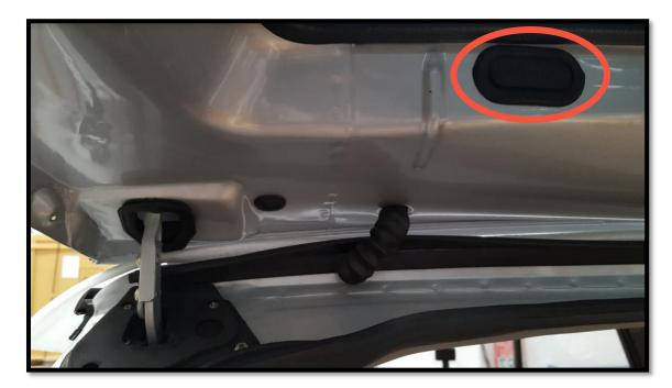
2. Pull out the wiring loom and disconnect wires. There is constant voltage so be careful and avoid the short circuit.
