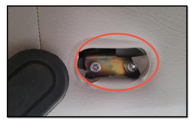
9. Take the hinge with the gas strut off the canopy.
