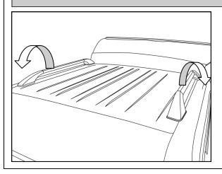
Remove the factory fitted plastic roof rails from the canopy by unclipping the screw covers and removing the securing screws. (These will not be reinstalled)
