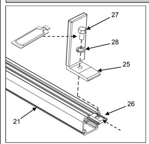
Slide a channel nut (26) into the end of the top profile of each cross bar (21).
