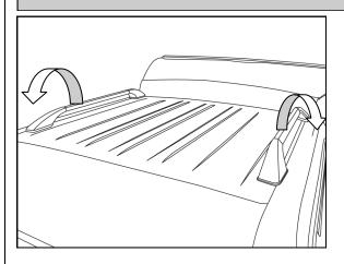
11. Remove the factory fitted plastic roof rails from the canopy by unclipping the screw covers and removing the securing screws. (These will not be reinstalled)
