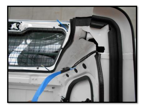
4. Remove the plate from rear door by unscrewing the three screws.
