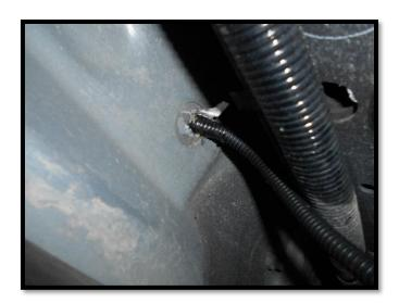
Alternatively, if there is no opening you can run the loom inside the vehicle to behind the back seat on the driver's side. There is a vent between the cabin and the tub you can run the loom through.
