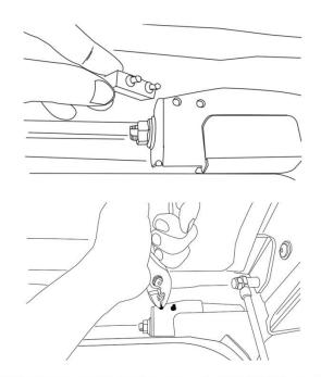
5. Attache spring pushing bracket (O) with the truck using original bolt (P). If the truck has stopping rubber, can put it back through hole (Q)
